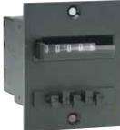
This unit is a highly versatile Pneumatic Predetermining Counter. It counts down from a preselected number and gives a pneumatic signal output when zero is reached. The output can then be used to actuate or initiate machine functions. The PC-3PM can be used in combination with pneumatic logic controls, limit switches, proximity switches, and similar controls.
